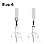
Fully insert the new wax guard so that it's flush with the top of the receiver, then pull the tool straight out.
